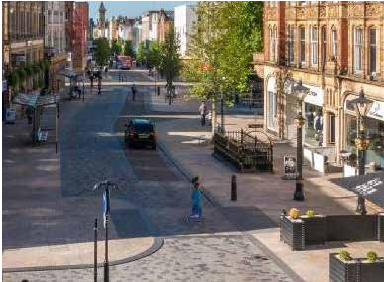
Figure 49: Subtle changes in materials to delineate separation of uses, with priority for pedestrians, Preston
